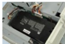
Battery • Type: Li-Ion 4S2P • Normal Voltage: 14.8V, 3800mAh • Backup: 100W/10min
