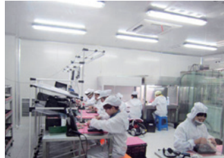
Control room particle measure result: Class 10000
