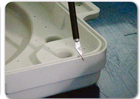
Deburring (Robot+Cutting tool)
