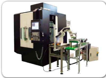
Loading / Unloading (CNC+Robot)
