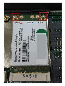
3. Attach the flat end of the antenna cable to the connector marked MAIN on the module and insert the other end of the cable with the connector tube into the antenna hole marked MAIN on the front panel of the computer.
