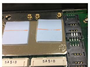
2. Insert the wireless module in the designated socket and tighten the two screws on the module.
