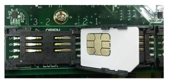
3. Push down the SIM card holder until the SIM card is secured in place.
