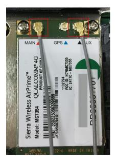
Refer to the following figure provided on the front panel to identify the antenna mounting holes for the wireless modules.
