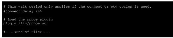
6. Add one of two files: /etc/ppp/options.eth0 or /etc/ppp/options.eth1. The choice depends on which LAN is connected to the ADSL modem. If you use LAN1 to connect to the ADSL modem, then add /etc/ppp/options.eth0. If you use LAN2 to connect to the ADSL modem, then add /etc/ppp/options.eth1. The file context is shown below:
