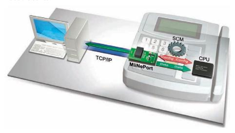
**EZPage:** Need a module that allows direct communication with the attached serial device? Use the MiiNePort E2's EZPage with Java Applet to create a visual webpage for configuring and communicating with the attached serial device.
