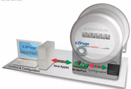
**AutoCFG (Auto Configuration)** saves time and effort when setting up the MiiNePort E2 one by one during the device production process.
