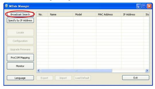
When the search is complete, every MGate MB3000 that is found on the LAN will appear in the window with MAC address and IP address. Simply select the one that you wish to configure.
