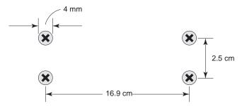
The head of each screw should be 6 mm or less in diameter, and the shaft should be 3 mm or less in diameter. Make sure to leave about 5 mm of space between the head and the wall.
