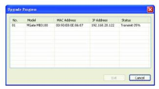
Once the firmware has been successfully written onto the unit, click Exit to close the Upgrade Firmware window. MGate Manager will automatically execute a Broadcast Search for all MGate MB3000 units on the LAN. Your MGate should reappear in the list of units.
