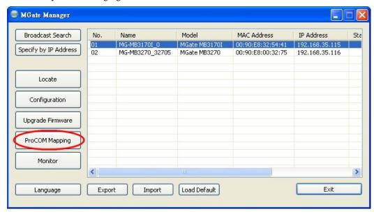
On the ProCOM mapping dialog box, you can map up to four ProCOM functions for each Modbus gateway to your PC's COM ports. The driver will generate virtual COM ports on your PC to connect to the selected MGate MB3000s over the network.
