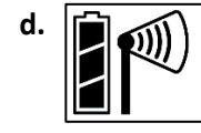
Once the mote has finished joining the network, the "x" icon is removed and the channel count on the station LCD increases by four (three for wind speed, wind direction, and gust speed, and one for the mote battery).
