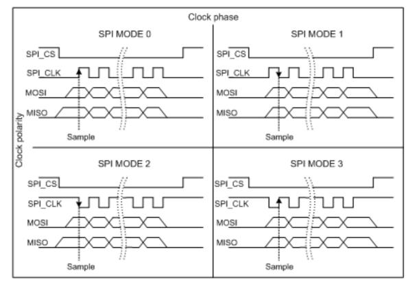
Figure 17.1: SPI modes selectable on SPI
