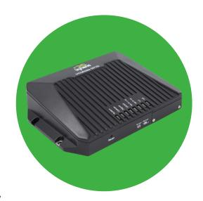
The InVehicle G710 4G LTE gateway provides high-speed and secure network access for vehicles and transportation services, including special-purpose, law enforcement, emergency, engineering and ambulance vehicles. The cloud-based fleet management platform provides continuous supervision for logistics management, asset tracking, mobile offices and government security works.
