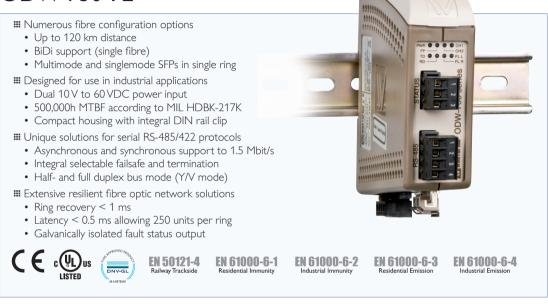
The ODW-730-F2 has been designed to allow the use of fibre optic cables on RS-422/485 networks. The design allows the use of a range of Westermo verified SFP (Small Form Pluggable) transceivers which can provide solutions with, for example, only a single fibre or distances up to 120 km. Both multidrop networks and redundant rings can be formed using a mixture of transceiver types.
