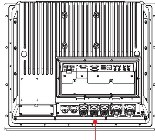
Connectors (must be installed by the user)
