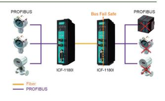
can automatically detect the baudrate of the PROFIBUS device and apply this baudrate directly. This is an extremely convenient feature. If necessary, baudrates can be set to a fixed value via DIP switches.
