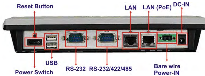
Figure 2-2: IOVU-751R-CE5/UX-R10 Peripheral Connectors
