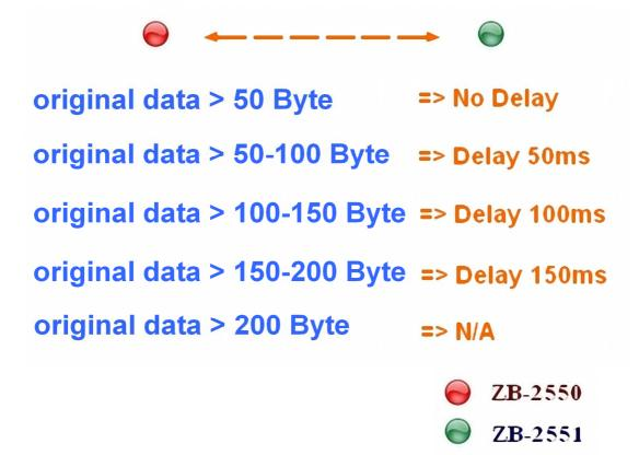
If original data size is **less than 50 Byte most of the time**, **Operating Mode Transparent** is the most suitable.
