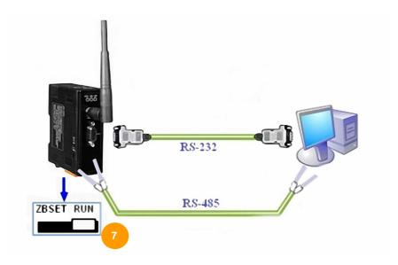
8. Click Default button to load factory default parameters if you want to load factory default setting of ZigBee Module
