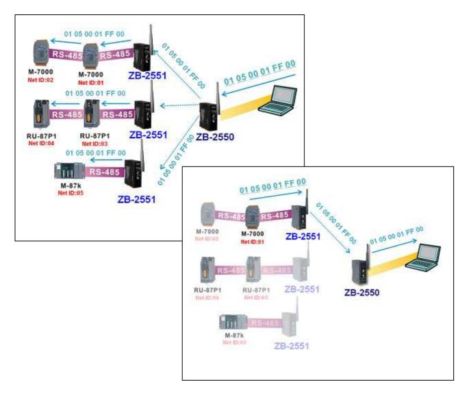
In some applications where the host controller needs to broadcast data to all RS-232/RS-485 devices and these devices receive data only (no response), you can also use this mode.
