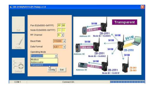
Modbus(Original data won't be broken down into small data) It is like Transparent mode. If original data size is greater than 50 Byte most of the time, Operating Mode Modbus is the most suitable. (Maximum original data size is 200 Byte. Original data must not more than 200 Byte, e.g. "\$01M" = 4 Byte)
