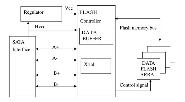
Figure 3: 2.5" SATA SSD Block Diagram
