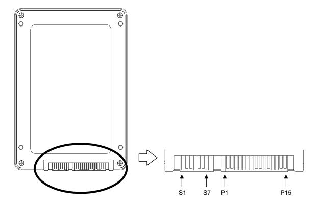
Figure 4: SATA Connector Pin Assignment
