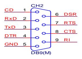
VXC-112A, VXC-182i (Male DB-9) Null Modem Cable Wiring
