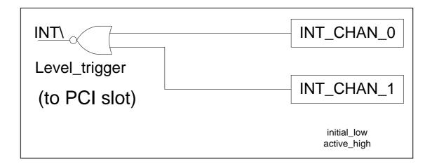
The interrupt output signal of the VXC card, **INT**, is Level-Trigger and Active\_Low. If INT\ generates a low\_pulse, the VXC card will send an interrupt signal to the PC only once. If INT\ is fixed in low\_level, the VXC card will send an interrupt signal to the PC continuously. Therefore, **INT\_CHAN\_0/1** must be controlled as a pulse\_type signal, which must normally be fixed in a low\_level state and should generate a high\_pulse when sending an interrupt signal to the PC.
