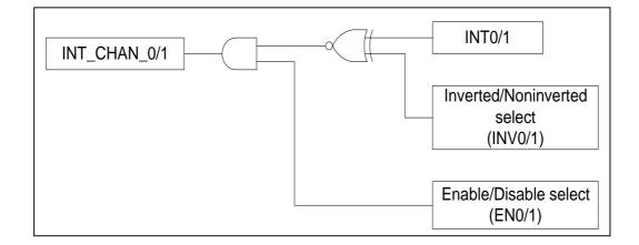
The INT\_CHAN\_0 and INT\_CHAN\_1 architecture is shown in the above figure. The only difference between INT0 and INT1 is that the INT\_CHAN\_0 signal source comes from the UART 0 interrupt output, and the INT\_CHAN\_1 signal source comes from the UART 1 interrupt output.
